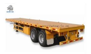
Ultratons'2 axles 20ft Flatbed Semi Trailer is a commonly seen model equipped with 2 pieces of semi-trailer axles for standard 20ft container. It can be modified according to customer's requirement.
